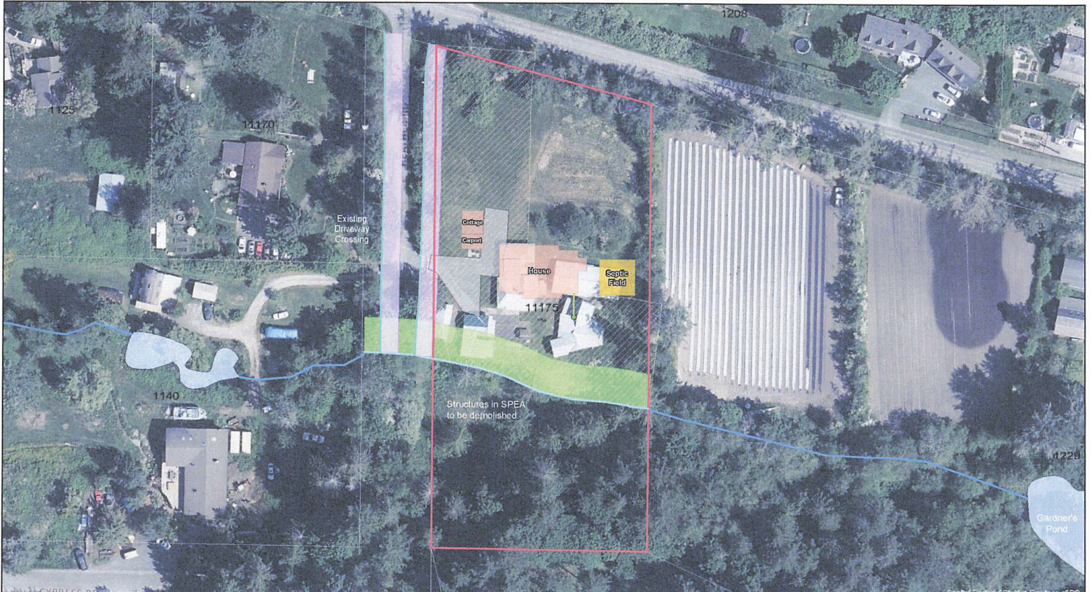
Site Plan and Riparian Assessment Area (RAA) and Zones of Sensitivity (ZOS)
